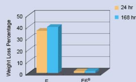
Weight loss comparison of E-glass and E6 ® fibers soaking in 10% H 2 SO 4 solution at 96°C after 24 hours and 168 hours
